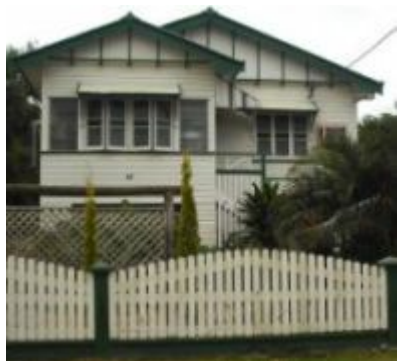
Figure 6.73 — Asymmetrical projecting building forms for a minimum 1.2m in depth (Burton Street)
