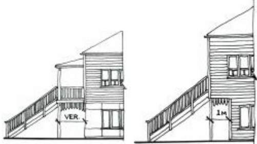
Figure 6.74 - Appropriate enclosures to the ground floor
